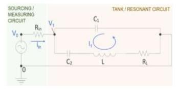
Figure 2.- Modified tank circuit sheme.
